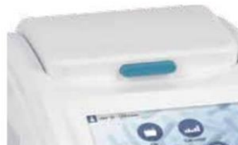
Clever hot lid elastic structure design adaptive to different height of tube
